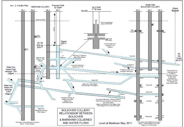
Figure 1: Schematic of the Markham colliery complex
