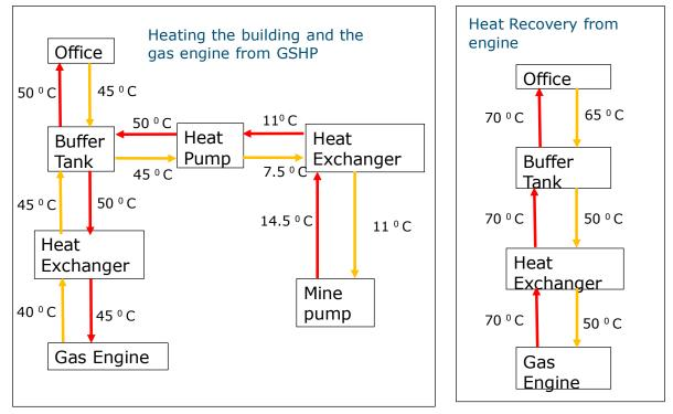
Figure 16: Schematic of the GSHP engine heating.
