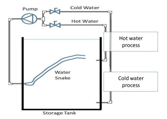
Figure 22: A schematic diagram of the automated experimental test rig.
