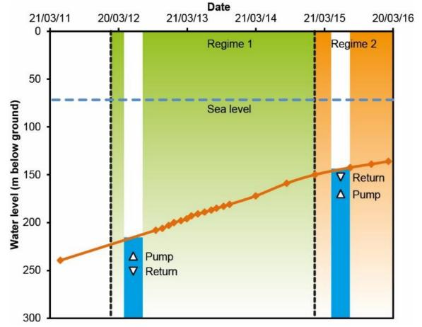
Figure 2: Schematic of the Markham No. 3 Shaft 'standing column' heat extraction arrangement, with rise in water level plotted ('Burnside, et al., 2016)
