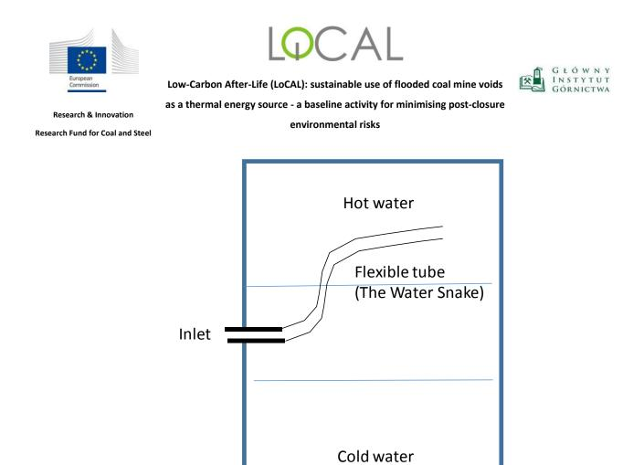
Figure 21: A schematic diagram that shows the movement of the water snake to the proper water layer that match the inlet water temperature.
