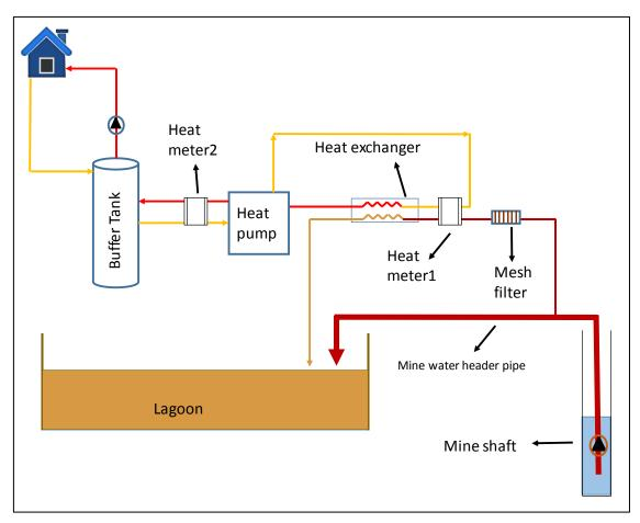
Figure 4: Schematic of the Markham system
