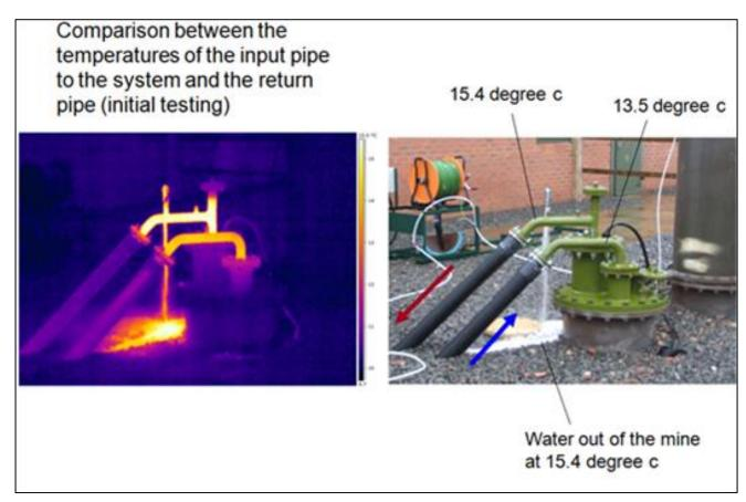
Figure 6: Thermographic image of mine water flow and return.
